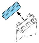
3. Remove the air filter element from the air filter housing.
